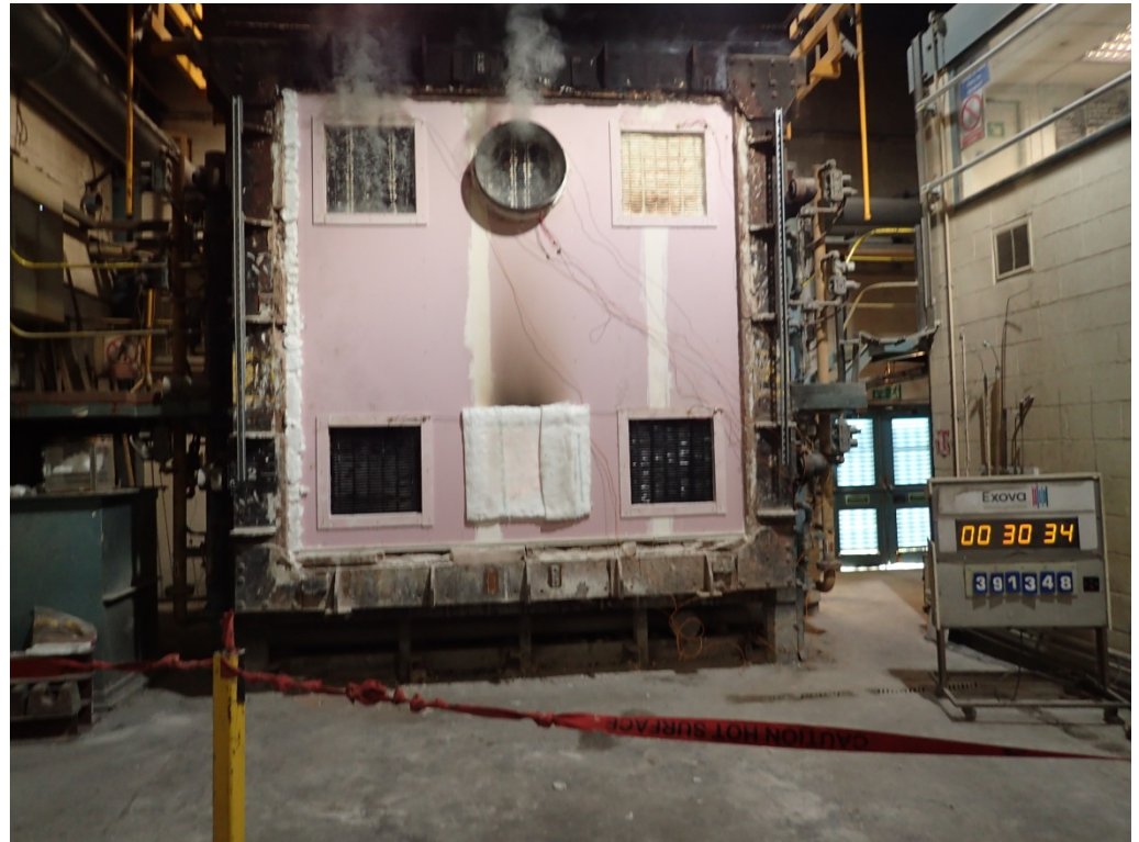
The unexposed face of the test constructions after a test duration of 30 minutes
