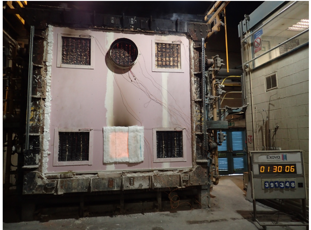
The unexposed face of the test constructions after a test duration of 90 minutes
