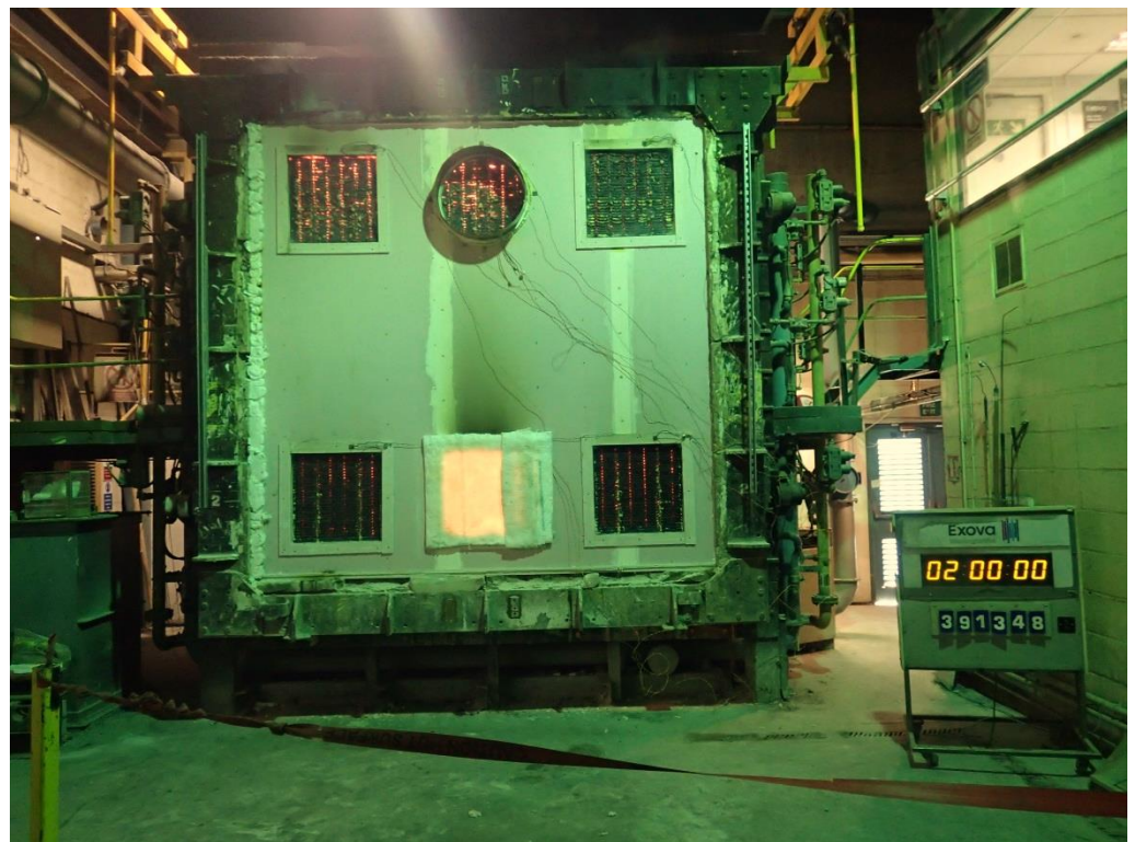
The unexposed face of the test constructions after a test duration of 120 minutes
