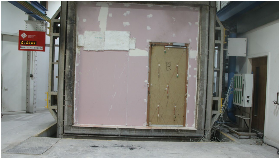
Figure 25 - The unexposed surface of the test construction after a test duration of 63 minutes
