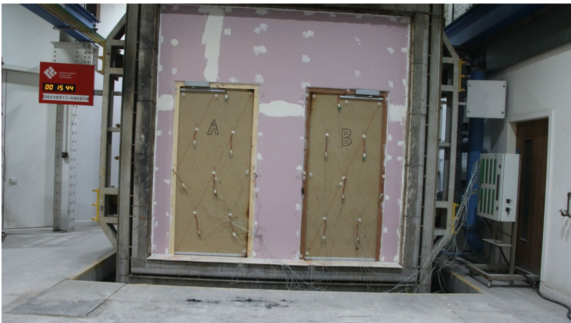
Figure 18 - The unexposed surface of the test construction after a test duration of 15 minutes
