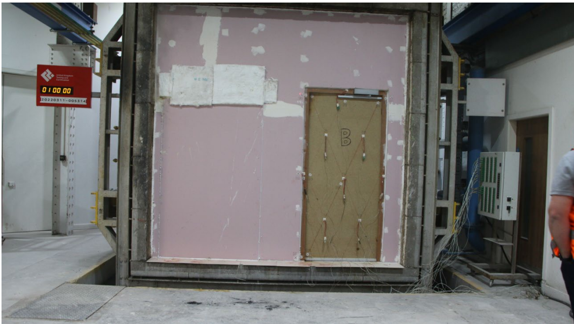
Figure 24 - The unexposed surface of the test construction after a test duration of 60 minutes
