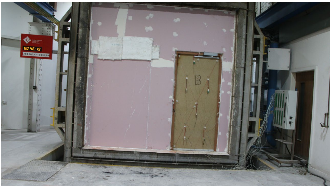
Figure 22 - The unexposed surface of the test construction after a test duration of 46 minutes
