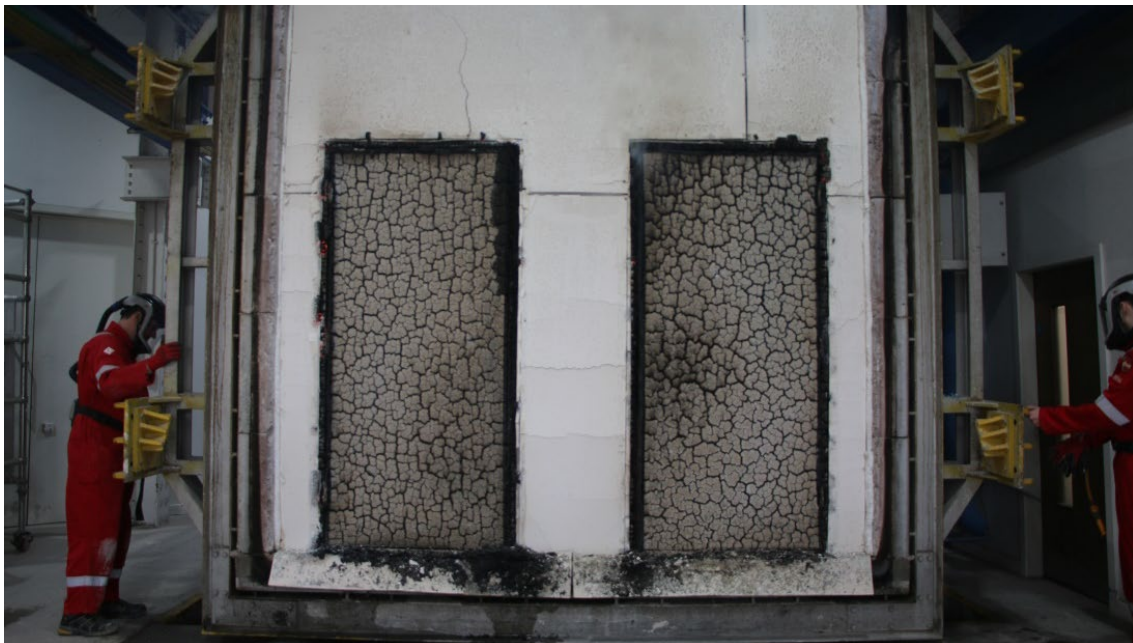
Figure 26 - The exposed surface of the test construction after the test was discontinued
