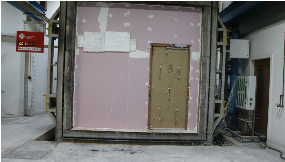
Figure 23 - The unexposed surface of the test construction after a test duration of 50 minutes
