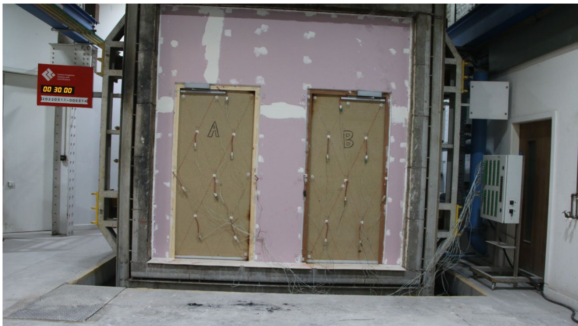
Figure 20 - The unexposed surface of the test construction after a test duration of 30 minutes
