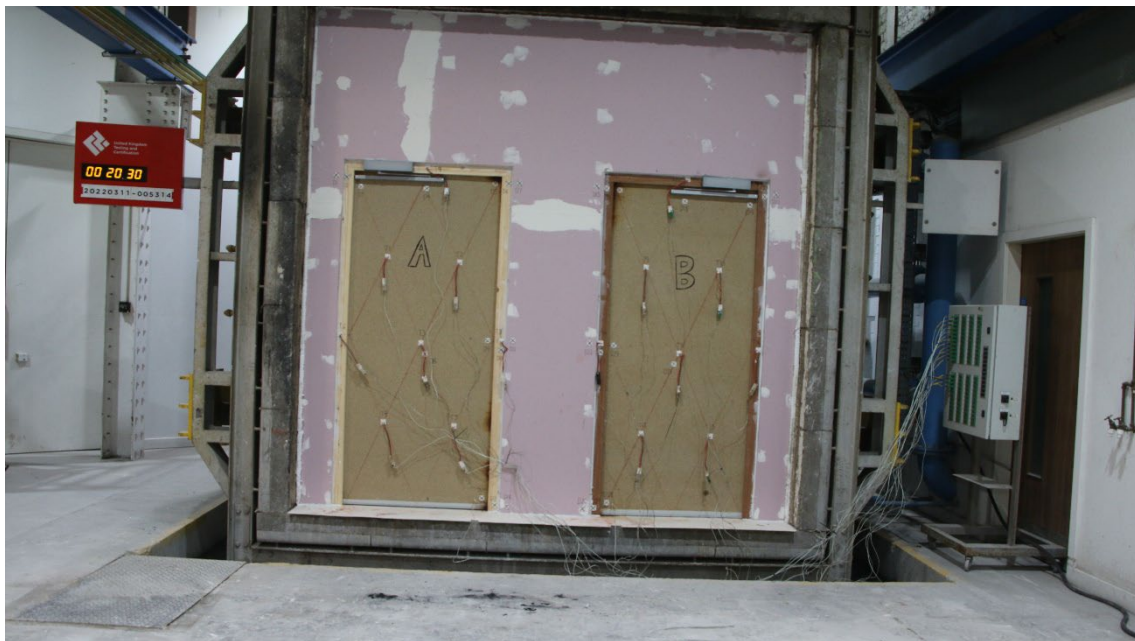
Figure 19 - The unexposed surface of the test construction after a test duration of 20 minutes
