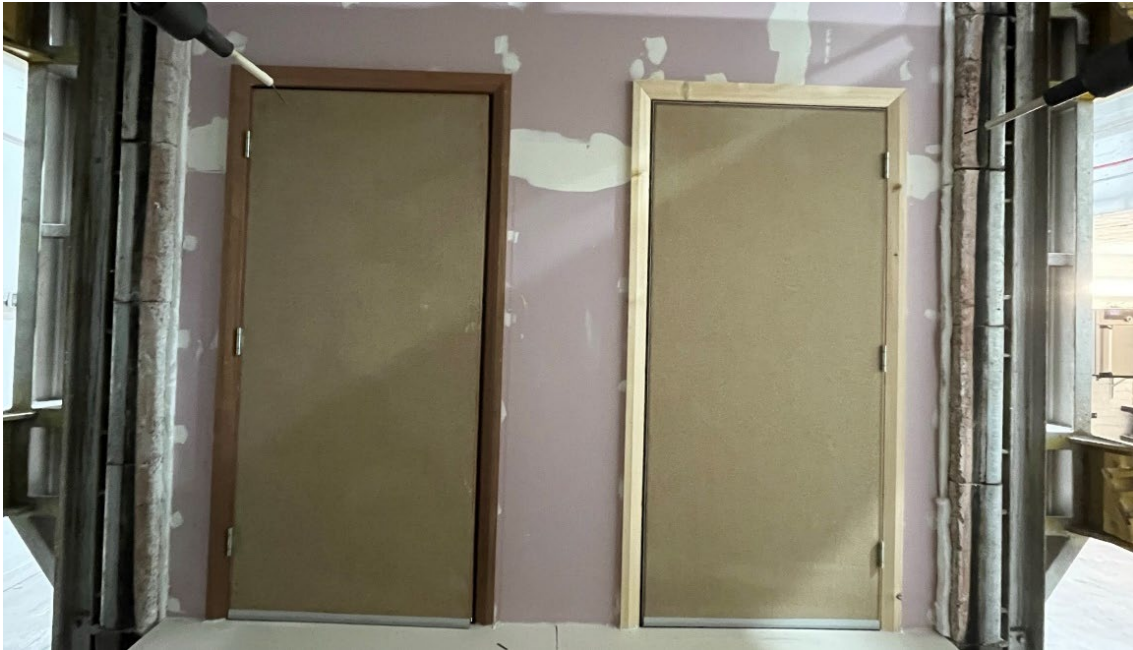
Figure 15 – The exposed surface of the test construction prior to commencement of the test
