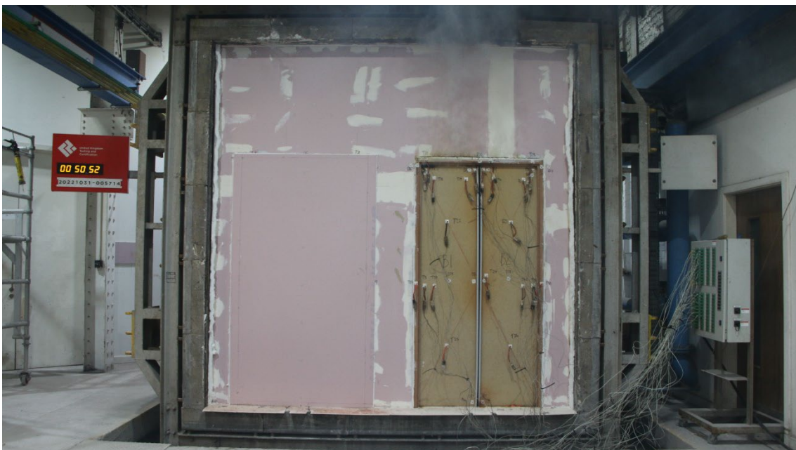
Figure 21 - The unexposed surface of the test construction after a test duration of 50 minutes
