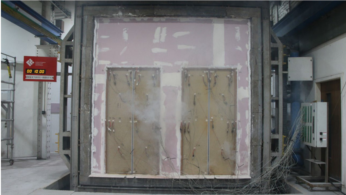
Figure 14 - The unexposed surface of the test construction after a test duration of 10 minutes
