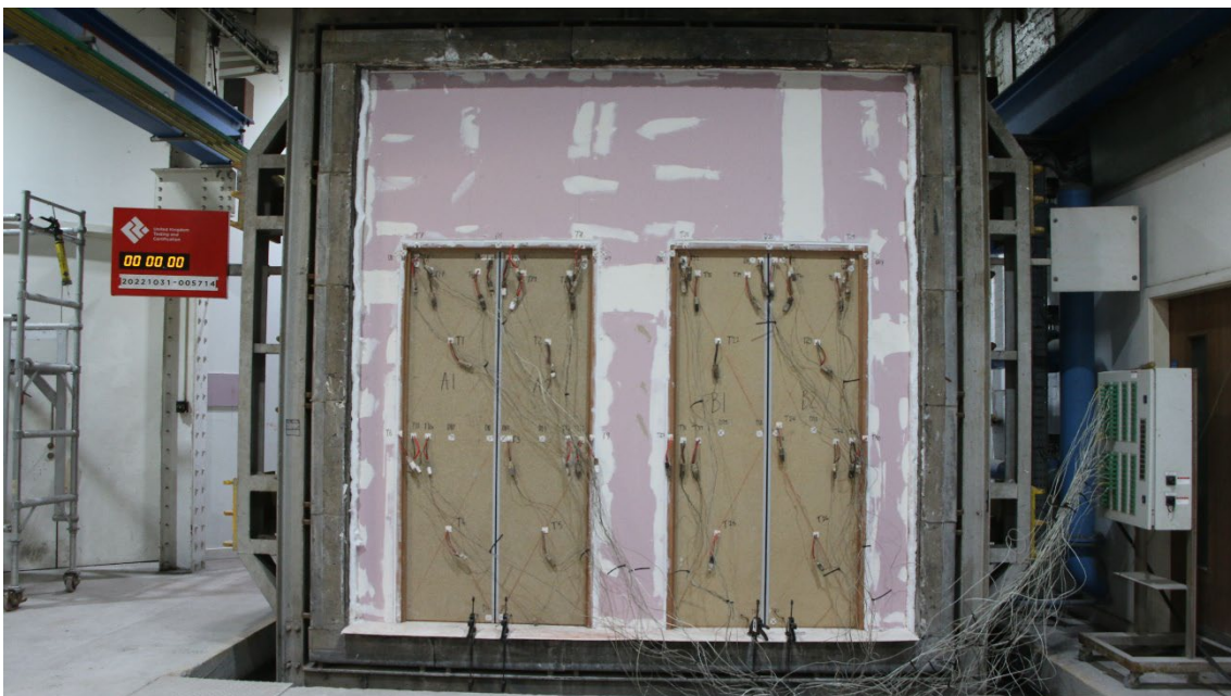
Figure 13 - The unexposed surface of the test construction prior to the commencement of the test
