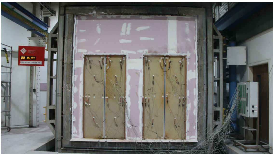
Figure 15 - The unexposed surface of the test construction after a test duration of 16 minutes
