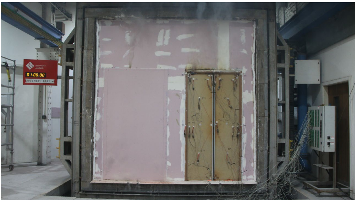
Figure 23 - The unexposed surface of the test construction after a test duration of 60 minutes
