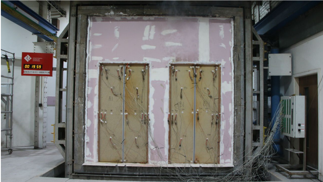
Figure 16 - The unexposed surface of the test construction after a test duration of 19 minutes
