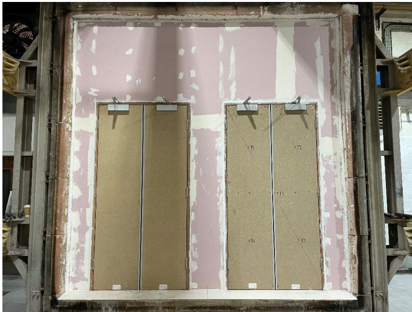
Figure 12 – The exposed surface of the test construction prior to commencement of the test
