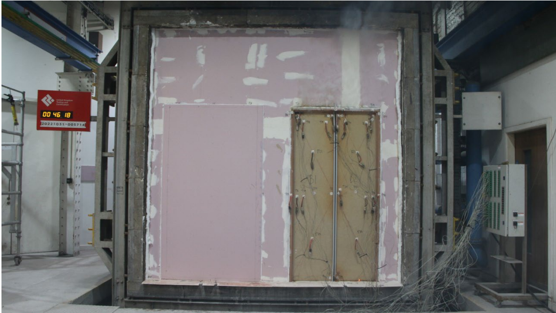
Figure 20 - The unexposed surface of the test construction after a test duration of 46 minutes
