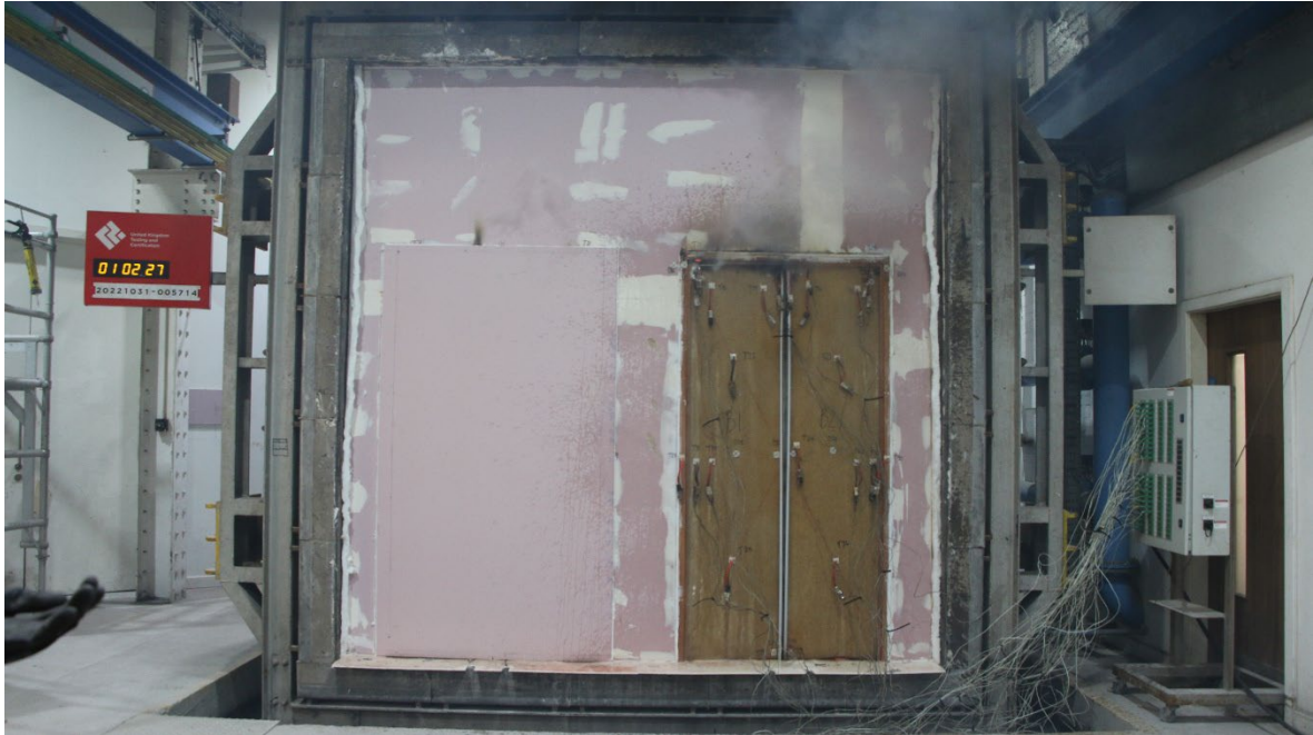
Figure 24 - The unexposed surface of the test construction after a test duration of 62 minutes
