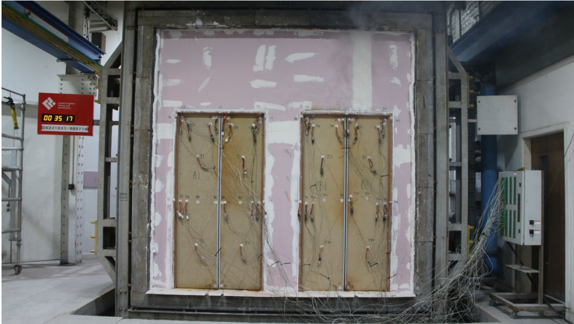
Figure 18 - The unexposed surface of the test construction after a test duration of 35 minutes
